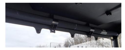
Small washer and lock nut on the inside.
