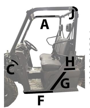
The hood will need to be raised to install the cab. Install the door kit and then lower the hood. You will need to pull back the front lower edge of the door kit (E) and pull the bungee down to latch the hood then reattach tab E.
