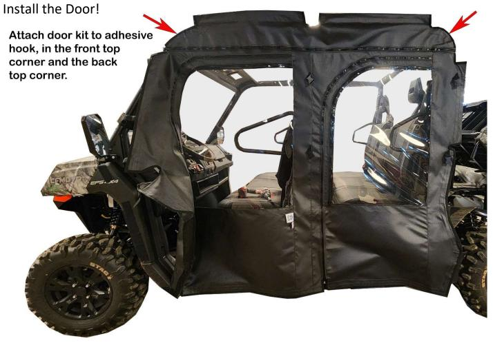
Wrap the back of the door kit around the rear roll bar.
