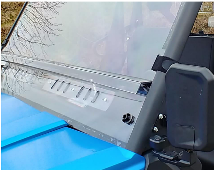
Figure 2: Shows how top portion of the windshield will set on the lower portion.
