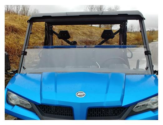
**Step 4:** Feed a strap into each of the slot holes. The strap should be inserted from the inside of the UTV with the loop side of the Velcro facing the middle of the UTV. Wrap the strap around the roll bar and feed it through the buckle. Pull the strap tight and adhere the hook end of the strap to the loop strap.
