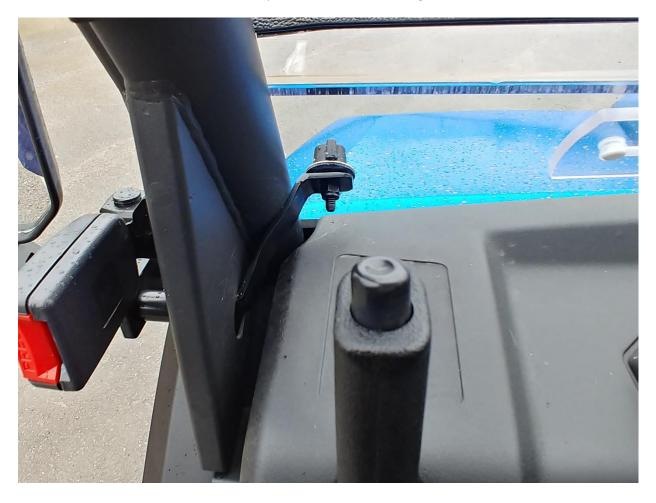
**Step 5:** The CC Clamps use the roll cage inset for connection. When installed properly, the back edge of the clamp attaches to the outside edge of the roll bar insert as shown below.
