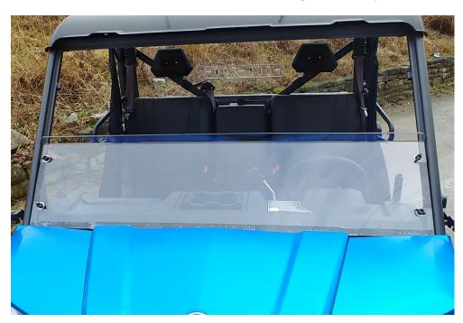
**Step 3:** Pull the protective paper from each bottom corner of the windshield to expose the holes for the bolts.
