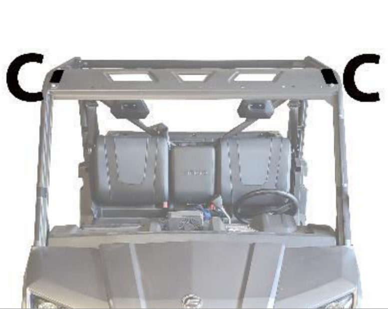
Figure 2: SHOWS PLACEMENT OF VELCRO STRIPS C.
