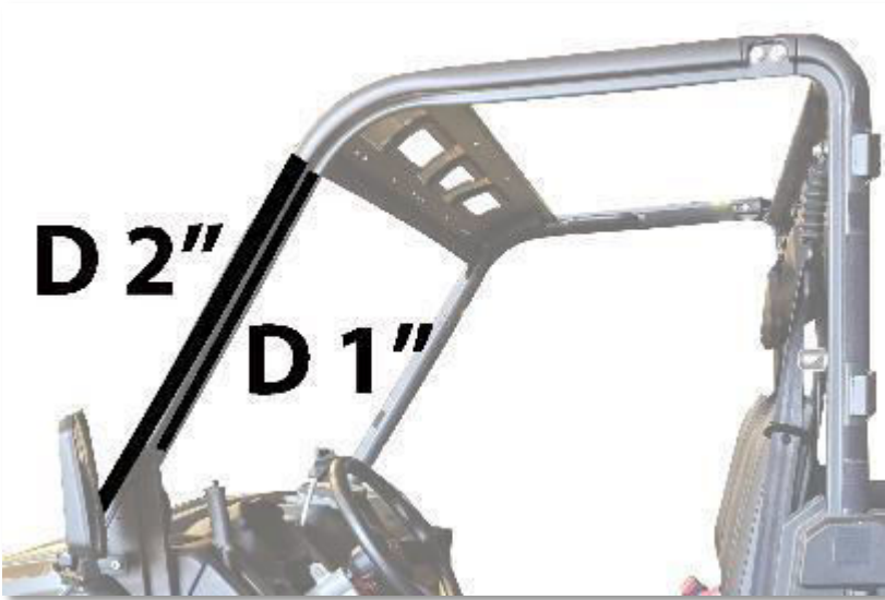
Figure 3: SHOWS PLACEMENT OF VELCRO STRIPS D.
