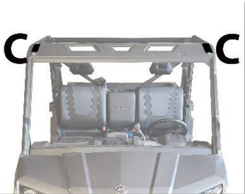
Figure 2: SHOWS PLACEMENT OF VELCRO STRIPS C.
