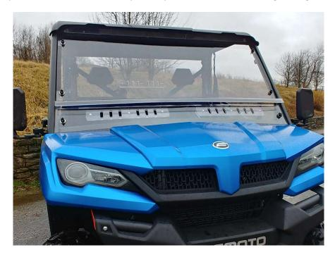
**Step 6:** When all clamps have been attached work your way around the windshield tightening all lock nuts.
