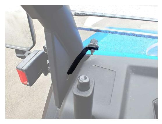
**Step 5:** Set top portion of the windshield in place with lower lip resting on the top of the bend in the lower portion of the windshield. Attach the C-Clamp in the same fashion as the metal bracket. Hand tighten only!
