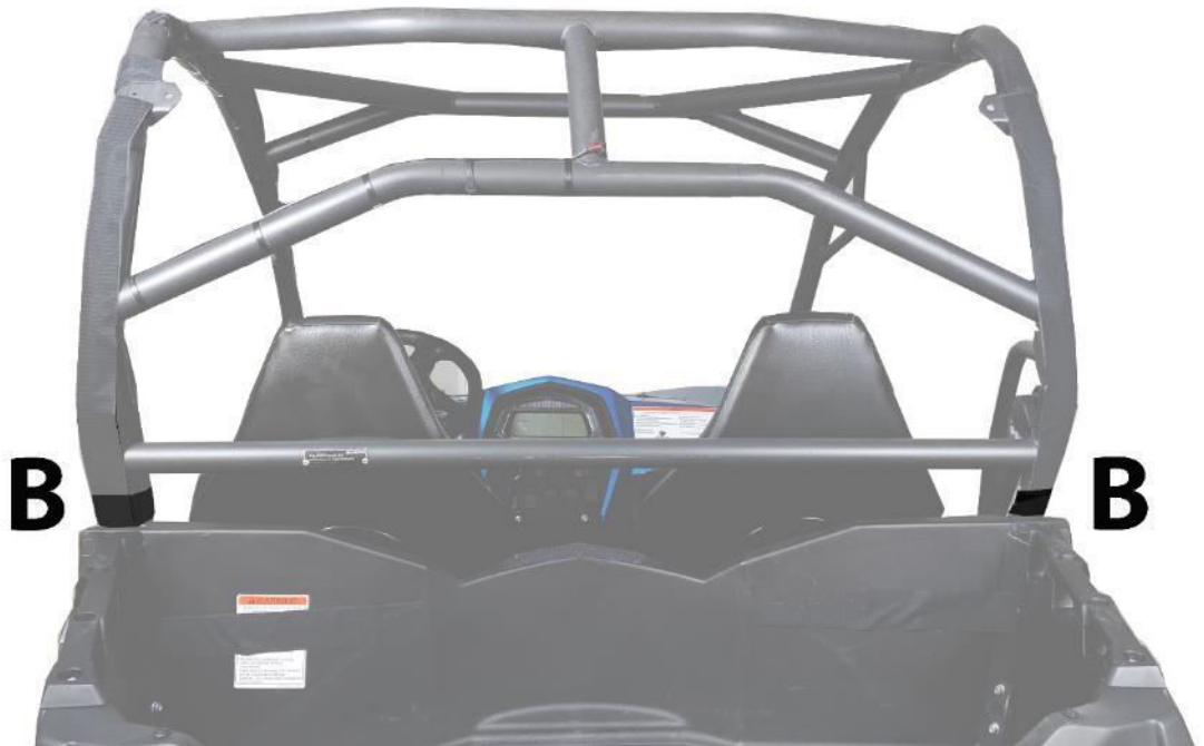
Figure 2: WRAP THESE VELCRO STRIPS AROUND THE ROLL BAR AND ATTACH DOUBLE-SIDED STRAPS.
