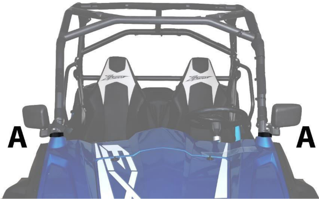
Figure 1: WRAP THESE VELCRO STRIPS AROUND THE ROLL BAR AND ATTACH DOUBLE-SIDED STRAP.
