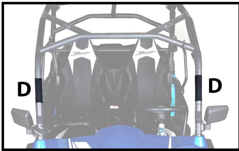
Figure 3: SHOWS PLACEMENT OF 7" VELCRO STRIPS (D).
