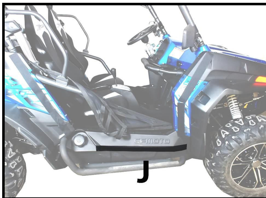
Figure 7: SHOWS PLACEMENT OF 31" VELCRO STRIP (J) YOU WILL PLACE AN IDENTICAL STRIP ON THE DRIVERS SIDE.
