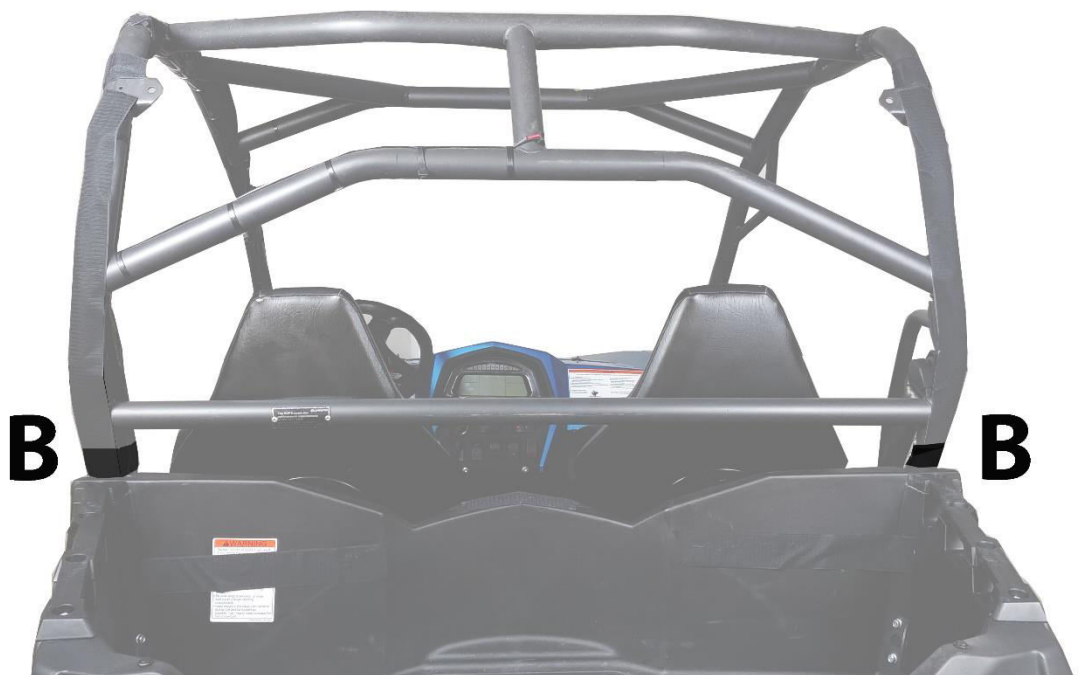
Figure 2: WRAP THESE VELCRO STRIPS AROUND THE ROLL BAR AND ATTACH DOUBLE-SIDED STRAPS.
