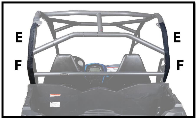
Figure 4: SHOWS PLACEMENT 21" VELCRO STRIPS (E) YOU CONNECT TABS E AND F TO STRIP E.
