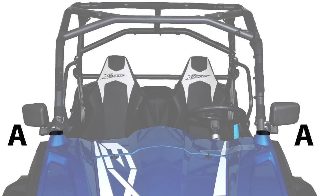
Figure 1: WRAP THESE VELCRO STRIPS AROUND THE ROLL BAR AND ATTACH DOUBLE-SIDED STRAP.
