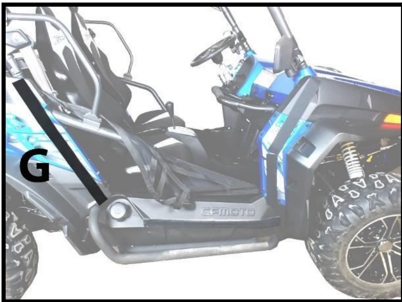
Figure 5: SHOWS PLACEMENT OF 34" VELCRO STRIPS (G) YOU WILL PLACE AN IDENTICAL STRIP ON THE DRIVERS SIDE.
