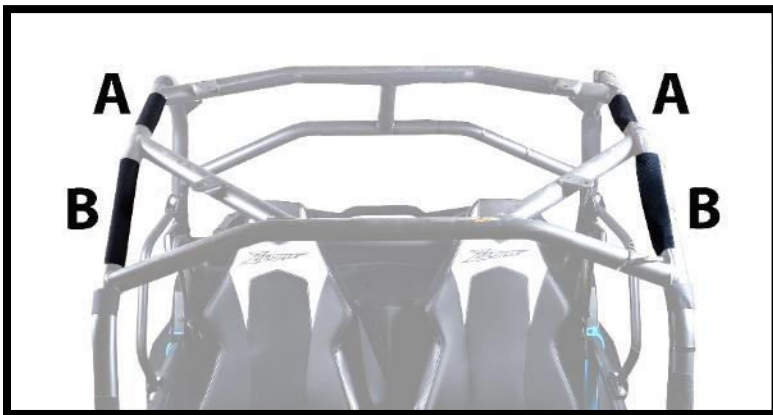
Figure 1: SHOWS PLACEMENT OF 6" VELCRO STRIPS (A) AND 10" VELCRO STRIPS (B) VELCRO TABS ON DOOR WILL WRAP OVER THE TOP OF THE ROLL BAR AND ATTACH TO ADHESIVE STRIP.
