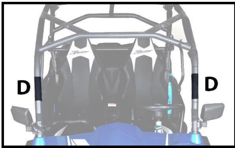
Figure 3: SHOWS PLACEMENT OF 7" VELCRO STRIPS (D).
