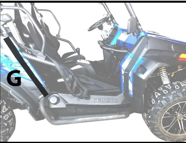
Figure 5: SHOWS PLACEMENT OF 34" VELCRO STRIPS (G) YOU WILL PLACE AN IDENTICAL STRIP ON THE DRIVERS SIDE.
