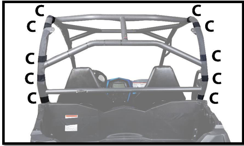
Figure 3: SHOWS POSITION OF 6" VELCRO STRIPS (C)
