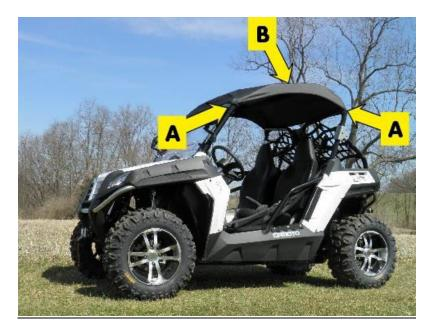
**Step 4:** Pull the top down tightly on the two front roll bars and two middle roll bars keeping the side seams aligned with the outside edge of the side roll bars. Wrap the double-sided straps around the attached Velcro strips.
