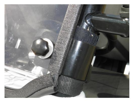
When installed correctly, the flat side of the clamp faces the windshield. The knob bolt with neoprene washer runs thru the clamp hole opening and is screwed into the clamp.
