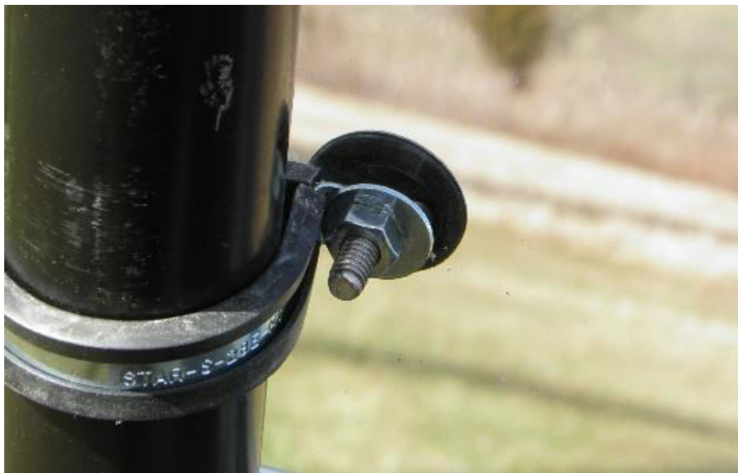
When installed correctly, the flat side of the clamp faces the windshield. The hex head bolt with neoprene washer runs thru the clamp hole opening and secured with a washer and nut on the back side.
