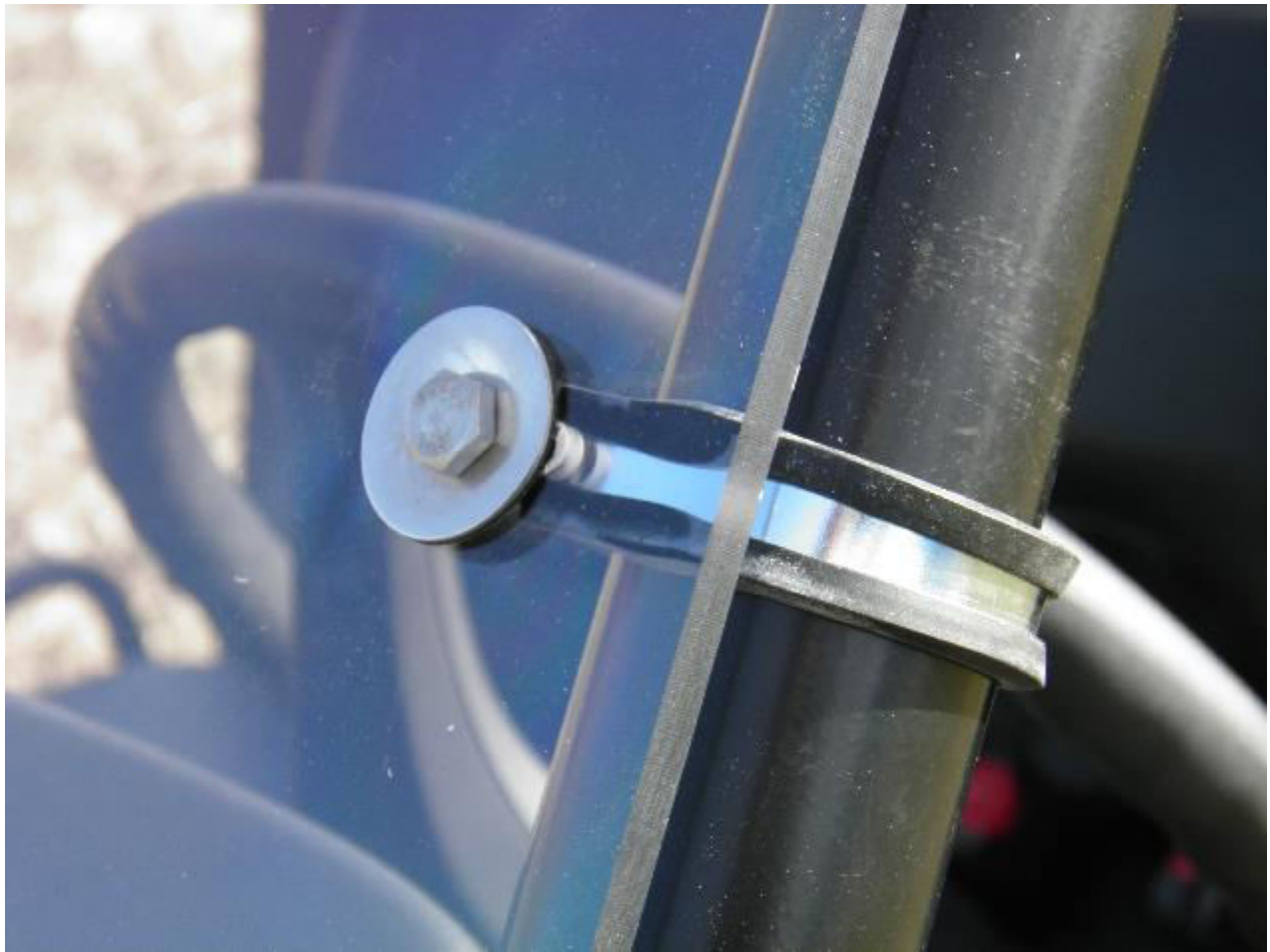
When installed correctly, the flat side of the clamp faces the windshield. The hex head bolt with neoprene washer runs thru the clamp hole opening and secured with a washer and nut on the back side.
