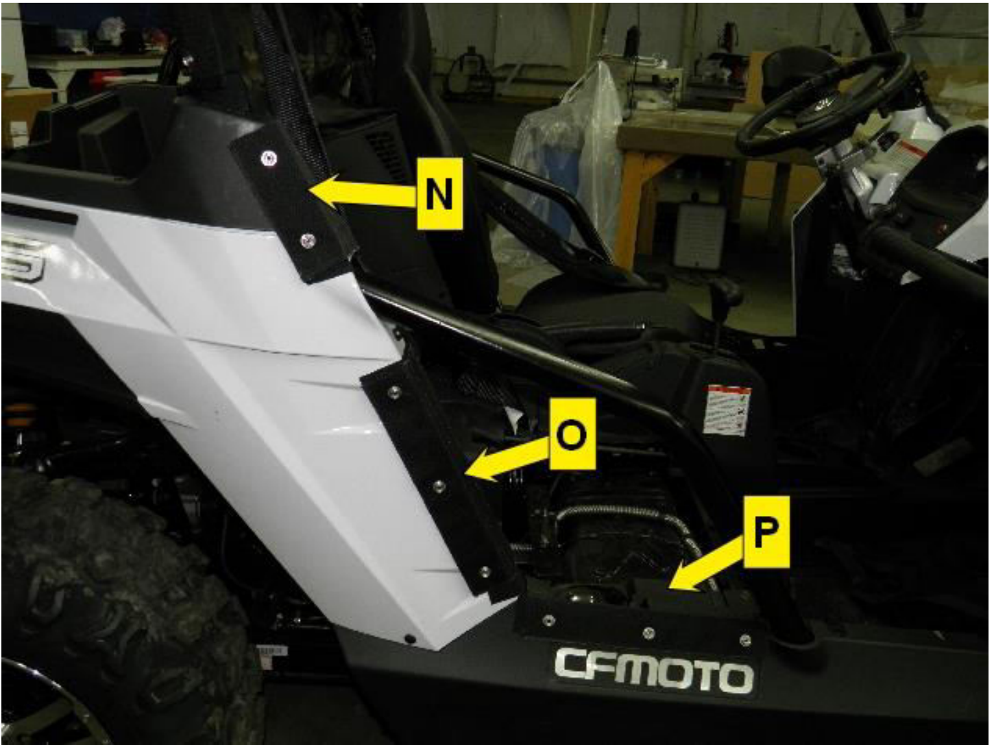
Installation of Snap Pads
