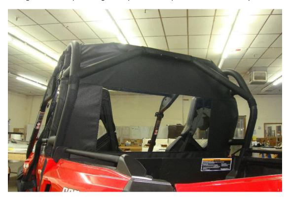
Note: The middle/top of the back panel wraps around the cross bar from the inside of the bar.
