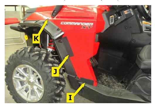
**Step 4:** After all adhesive Velcro strips are attached, with the exception of the front roll bars, begin attaching the doors to the frame.. Align and square the doors to the cab frame as you connect the Velcro strips.
