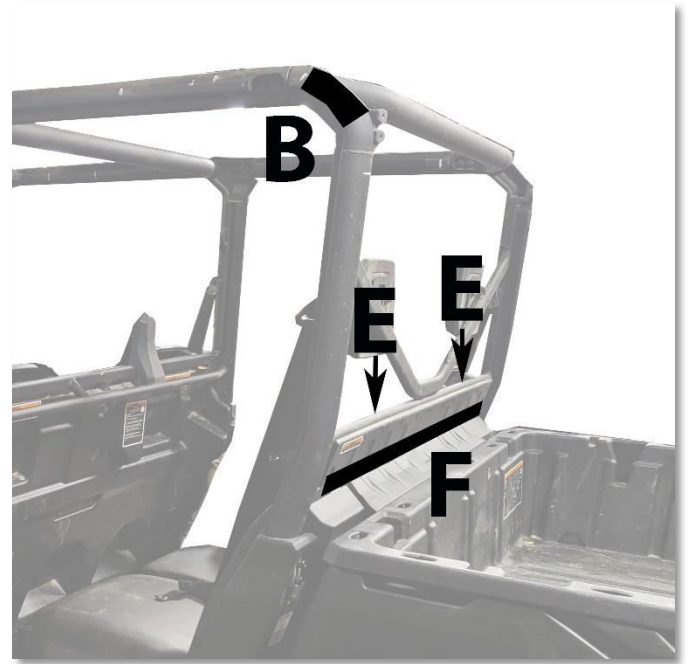
Figure 2: the double sided straps associated with strip B will wrap around the roll bar. Tabs E will fold over the back of the seat and attach in between the seat and the rear frame.
