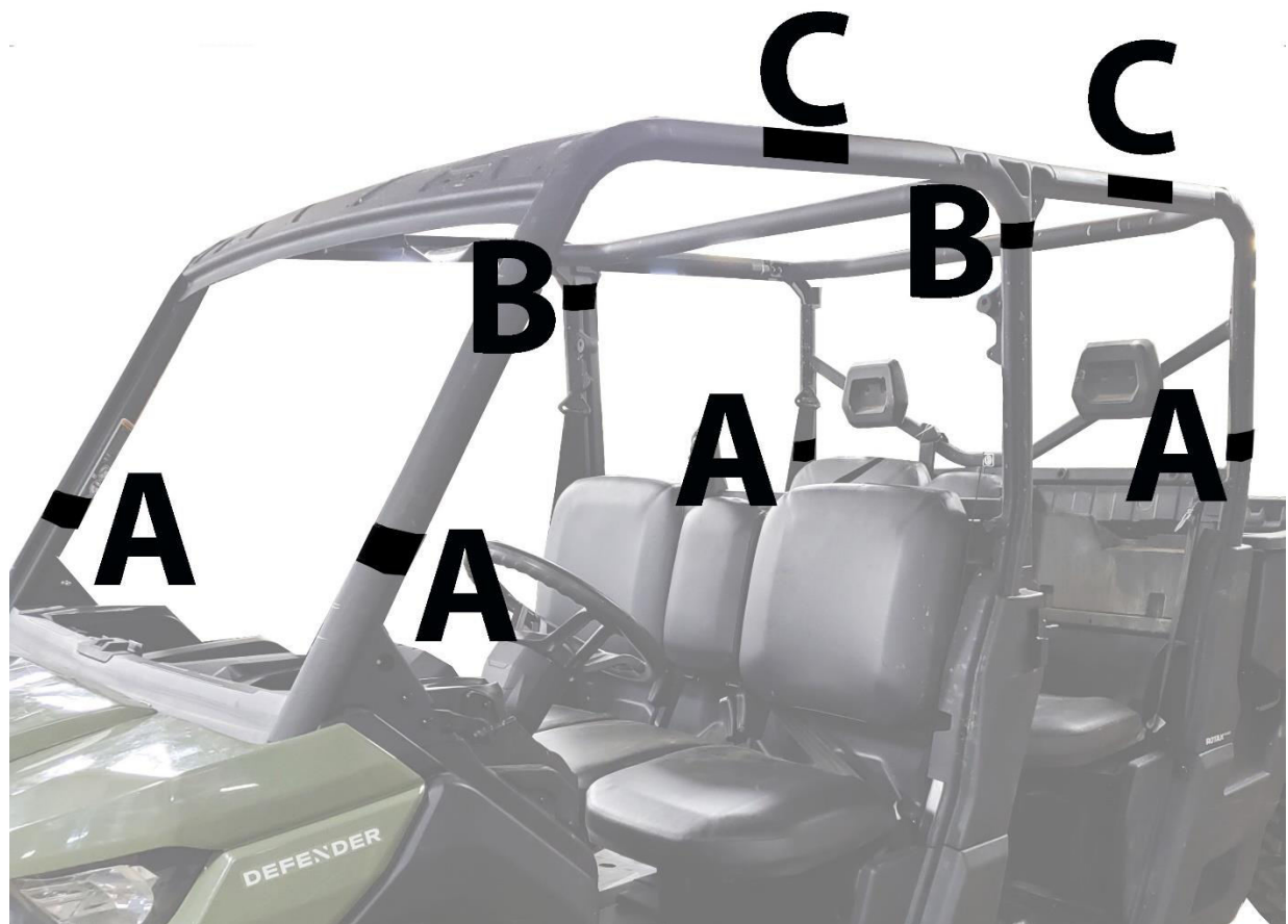
Figure 1: WRAP THESE VELCRO STRIPS AROUND THE ROLL BAR AND ATTACH DOUBLE-SIDED STRAP.
