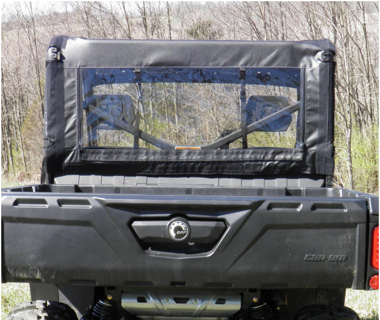
Figure 1: Align the top of the back panel up in the center of the roll bar. Wrap tabs C around the side of the roll bar and attach to strip C. D will wrap around the roll bar.
