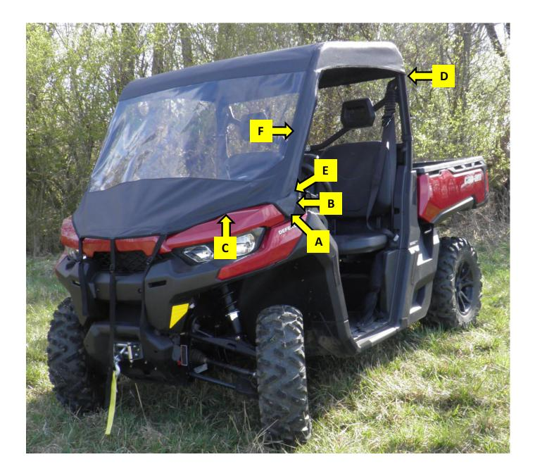
**Step 3:** After all adhesive hook strips are attached, begin attaching the enclosure to the cab frame. As you attach the hook and loop, square each panel to the frame. <u>PLEASE NOTE, FOR MAXIMUM ADHESION, ALLOW THE ADHESIVE</u> <u>HOOK TO ADHERE TO THE FRAME FOR 24 HOURS BEFORE PULLING AGAINST THE HOOK WITH THE LOOP STRIPS.</u>
