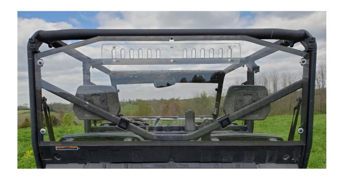
**Step 4:** As each clamp is placed into position, insert a hex head bolt thru a neoprene washer. Insert the bolt thru the back panel and thru the corresponding clamp. Insert a flat washer and lock nut onto the bolt. Only hand tighten at this time.
