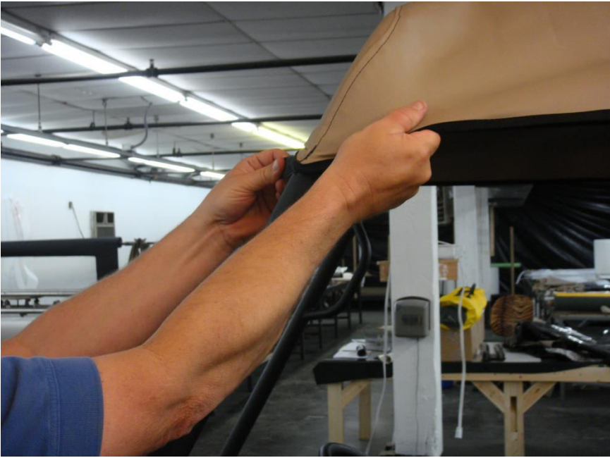
Figure 4.1 - Attach front and rear Enclosure Velcro tabs to installed Velcro strips
