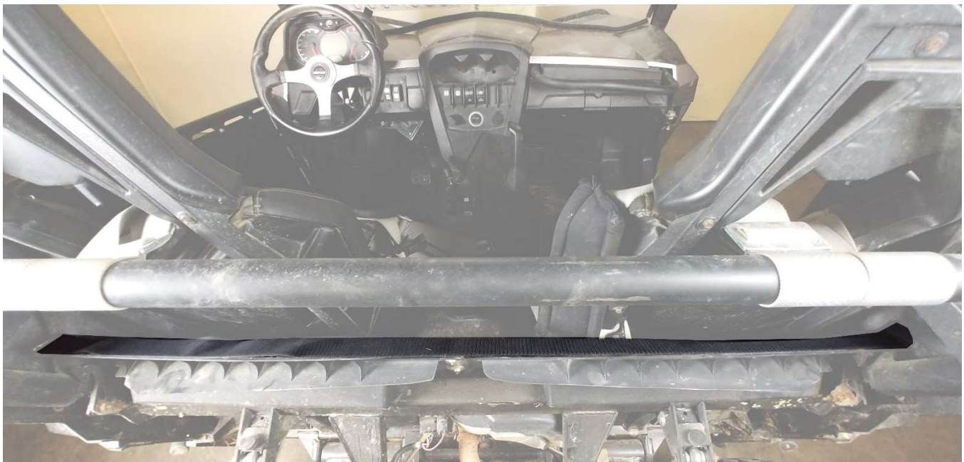
Figure 1: Shows placement of long piece of Velcro for the bottom of the fabric panel. The adhesive Velcro is installed on the inside of the cab.
