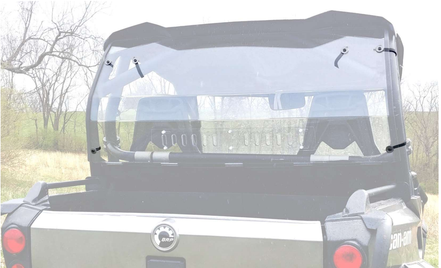
Figure 1: Shows placement and position of Loop Clamps.
