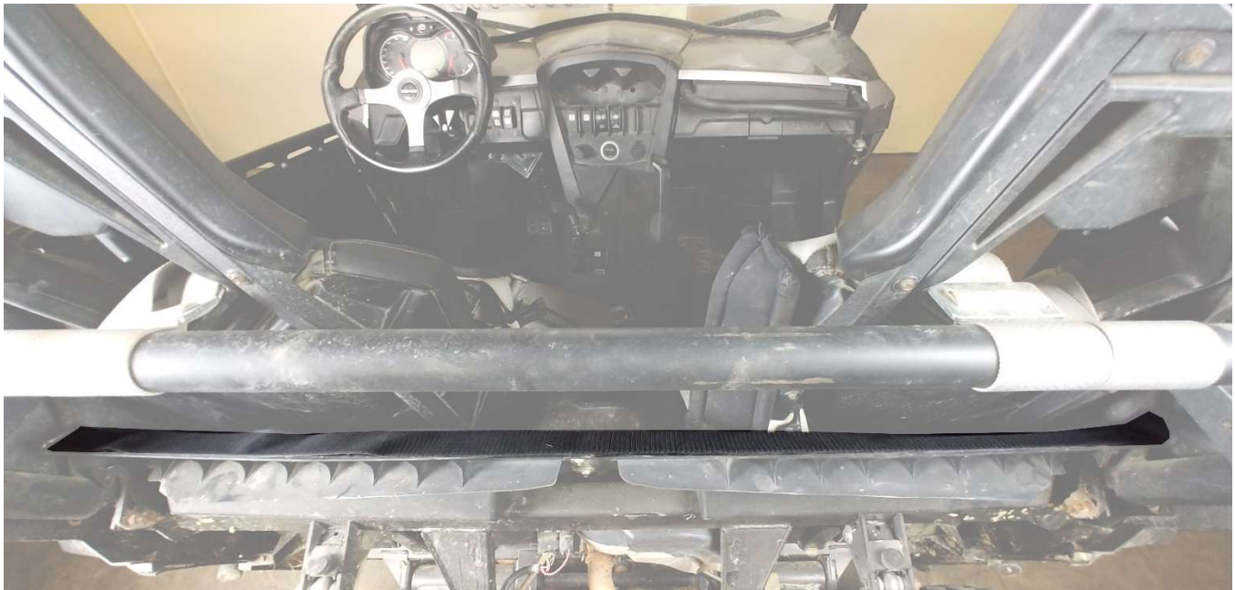
Figure 2: Shows placement of long piece of Velcro for the bottom of the fabric panel. The adhesive Velcro is installed on the inside of the cab.
