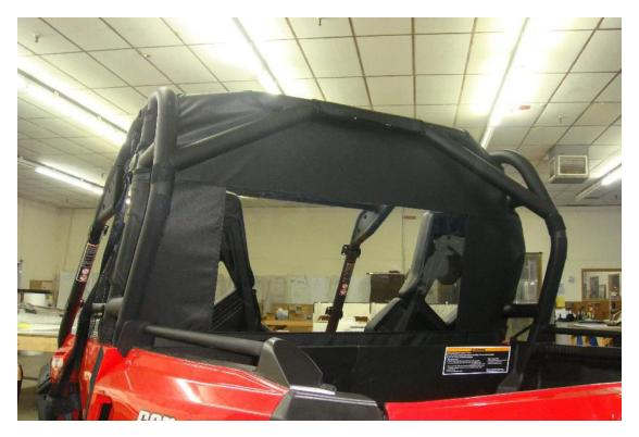
Note: The middle/top of the back panel wraps around the cross bar from the inside of the bar.
