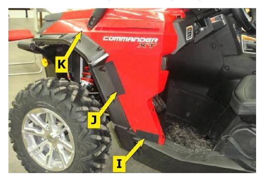
**Step 4:** After all adhesive Velcro strips are attached, with the exception of the front roll bars, begin attaching the doors to the frame.. Align and square the doors to the cab frame as you connect the Velcro strips.
