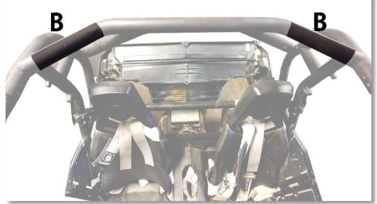
Figure 2: SHOWS POSITION OF 8" VELCRO STRIPS (B), TABS WILL WRAP AROUND THE TOP OF THE UTV AND ATTACH TO THE INSIDE OF THE CAB
