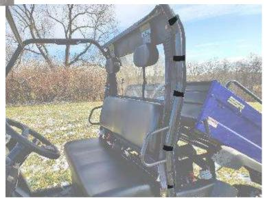
Pictures show the sewn on Velcro tabs and straps that correspond to the Velcro chart.
