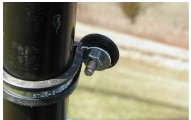
**Step 4:** When satisfied that the windshield is positioned properly, tighten the nuts on each clamp.
