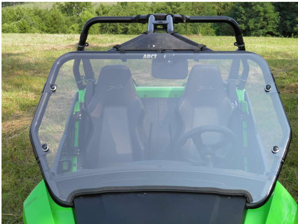
Figure 2.2 - place windshield so that the bottom center is approx. \frac{1}{4} " above the vehicle hood
