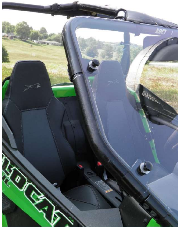
Figure 2.1 - Center Windshield between roll bar so that edges are in the center of the front Roll Bar posts
