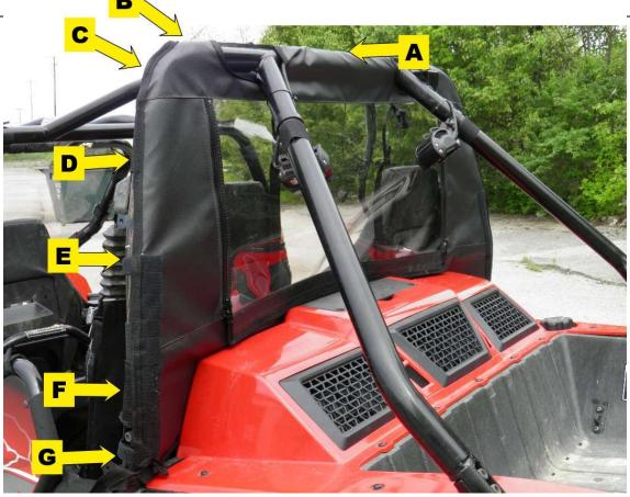
**Step 3:** Drape the windshield/top over the cab frame. Note, the 5" webbing/loop tab is located in the FRONT visor. The two double-sided strap are on the rear visor. The top attaches to the cab frame with tension straps. Attach the adhesive hook strips per the table and pictures below.
