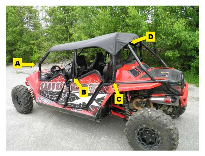
**Step 2:** Place Top Cap loosely on top of the vehicle Roll Bar Cage making sure the Enclosure front visor is facing toward the front of the vehicle. Pull the enclosure downward at each Roll Bar post upright to position the Enclosure snug to the Roll Bar Cab frame.
