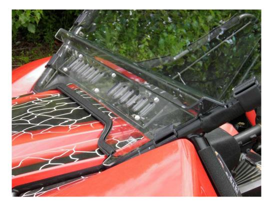
**Step 7:** Repeat Step 4 for each of the strap slots in the upper windshield section.
