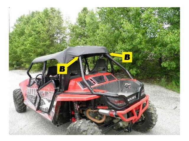
**Step 4:** Align the top to the cab frame as needed. When properly aligned, pull the loose strap on the tension straps to tighten the top to the frame. Work your way around the Wildcat. Little adjustments to each as you go around are best.
