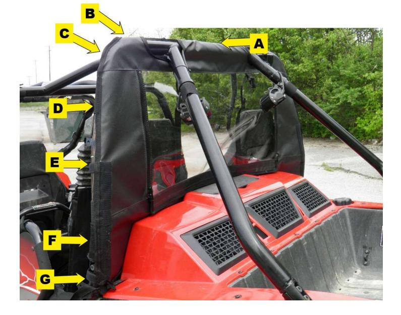
**Step 3:** Drape the windshield/top/doors over the cab frame. Note, the 5" webbing/loop tab is located in the FRONT visor. The two double-sided strap are on the rear visor. The top attaches to the cab frame with tension straps. Attach the adhesive hook strips per the table and pictures below.
