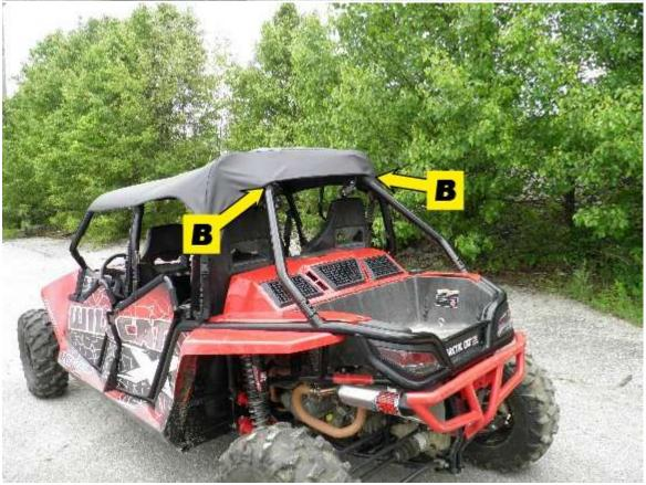
**Step 3:** Align the top to the cab frame as needed. When properly aligned, pull the loose strap on the tension straps to tighten the top to the frame. Work your way around the Wildcat. Little adjustments to each as you go around are best.
