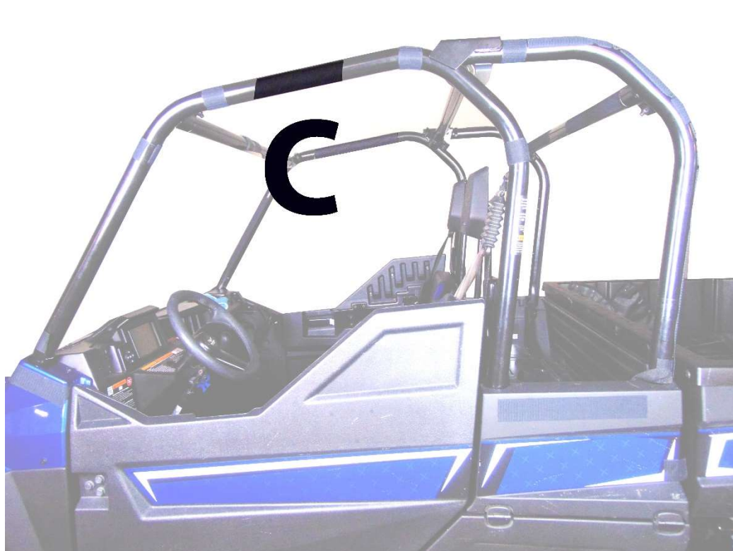
Figure 1: Place horizontally on the side roll bar, pull the tab on the roll bar over and around the top of the machine and stick to the adhesive Velcro.
