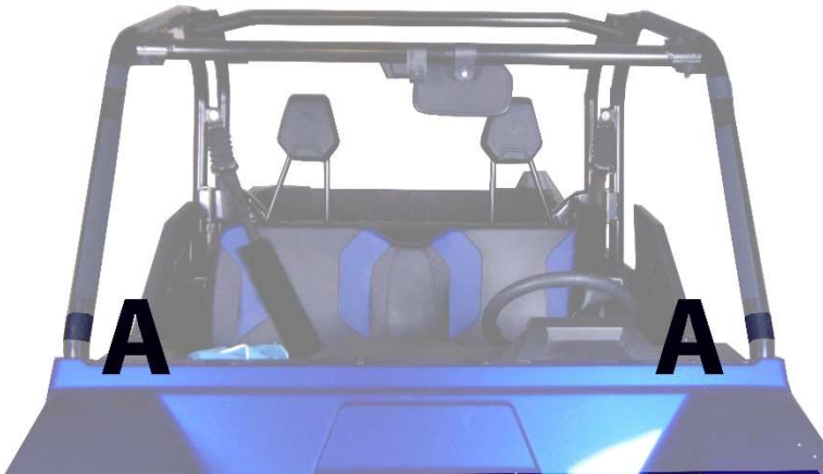
Figure 1: WRAP THESE VELCRO STRIPS AROUND THE ROLL BAR AND ATTACH DOUBLE-SIDED STRAP.
