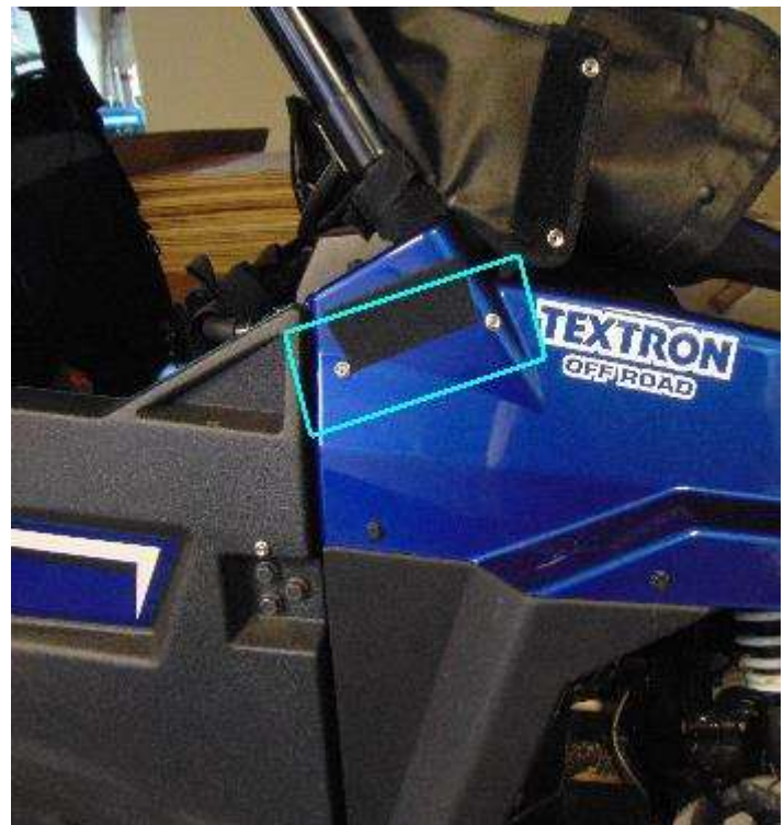
Figure 19: Install these snaps on the outside of the UTV.
