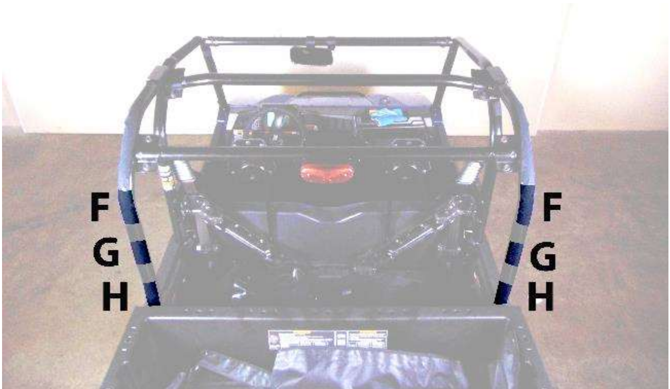
Figure 6: Shows placement of Velcro on the back panel, if you only purchased a door kit then you will place this strip on the roll bars from the top all the way down the back of the roll bars. If you have a back panel you will not need this Velcro. If you have a lexan back panel, the adhesive Velcro is optional, the lexan back panel will go over the door panels Velcro tabs, tightening the Lexan back panel into place will hold your doors to the UTV frame.
