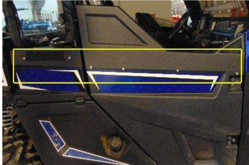
Figure 13: After installing the doors on the UTV you can then use the female end of the snaps attached to the door kit to determine the best spot for male end on the UTV. Mark the area on which you will install your snap, use a Phillips head screw driver to twist it into place.
