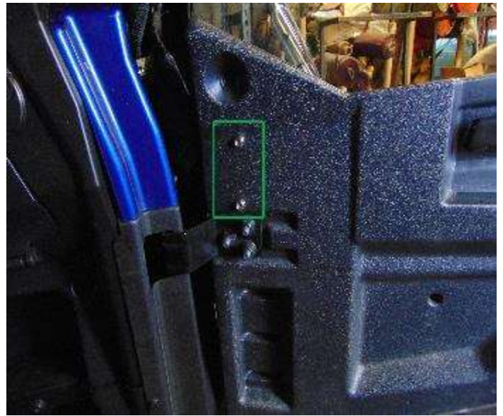
Figure 17: The photo above shows the general area on the inside of the factory door on which the male snaps should be placed. Remember to use the soft door as a guide when installing the snaps.
