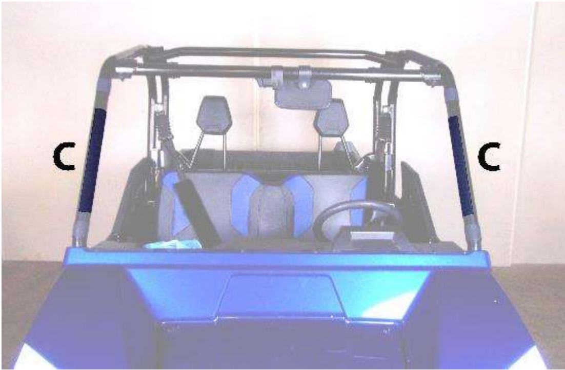
Figure 3: Shows placement of 14" Velcro strips C.
