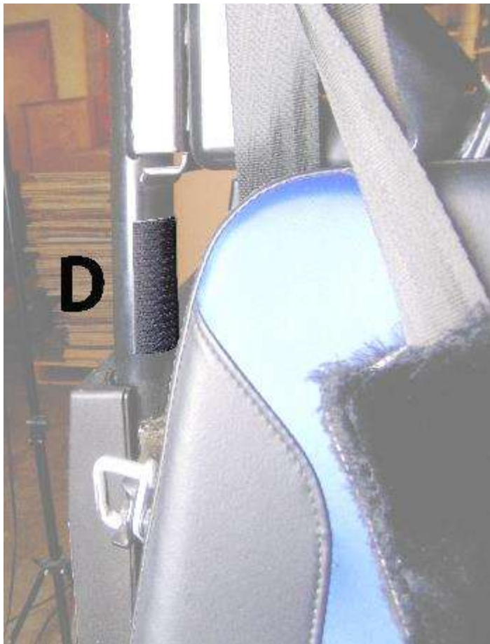
Figure 4: Shows placement of 4" Velcro strip D. You will install a Velcro strips in the same position on the opposite side of the UTV.
