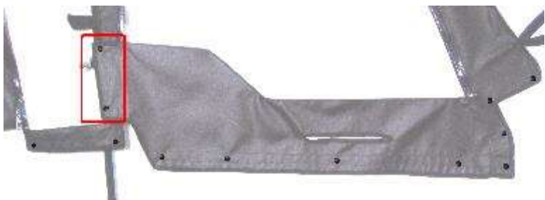
Figure 14: This flap on your door kit will wrap around to the inside of the door.
