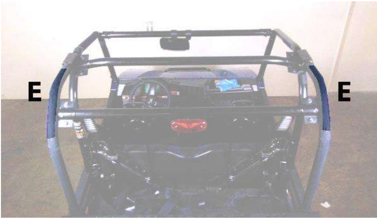
Figure 5: Shows placement of 16" Velcro strips E. These strips are installed on the top back roll bar extending down the curve.
