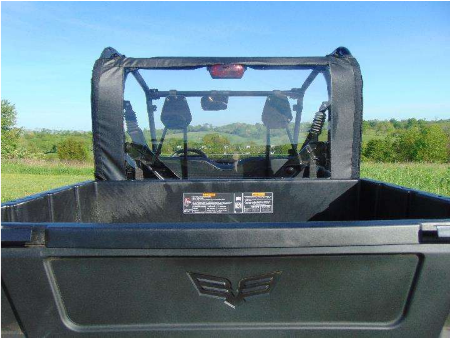
Figure 7: Upon completion of installation your back panel should be tight across the back of the UTV.
