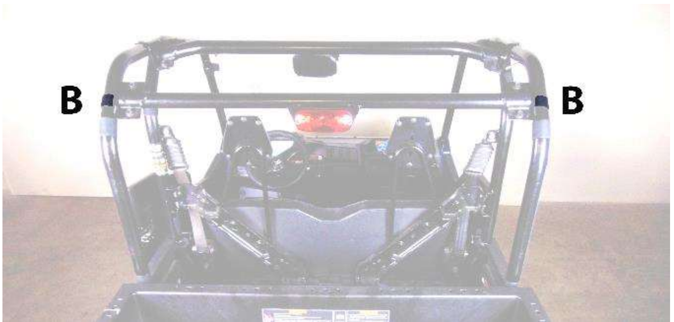
Figure 2: Shows placement of 3" Velcro strips B.
