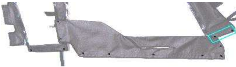
Figure 18: The snaps outlined in this photo will connect to snaps installed on the outside of the machine.
