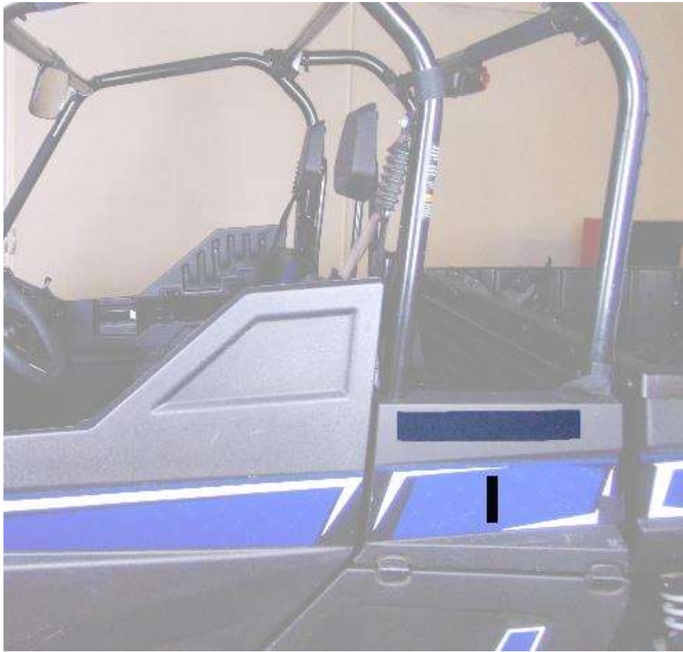
Figure 7: Shows placement of 9" Velcro strip I.
