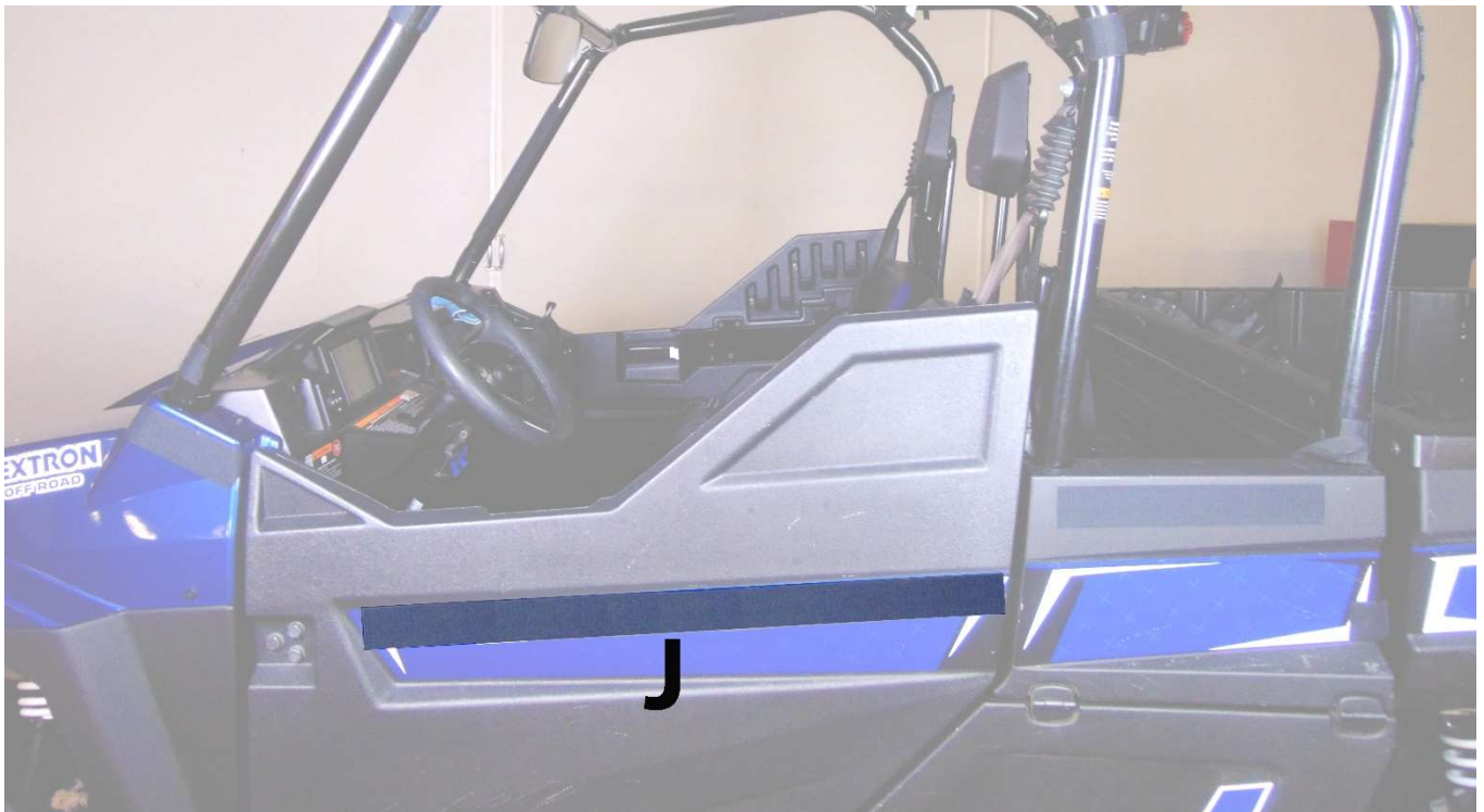
Figure 8: WARNING! Attaching this strip of adhesive Velcro may damage the decals when removed. Attach horizontally to factory door, place an identical strip on the passenger side.
