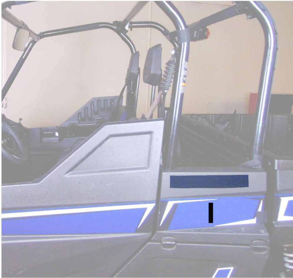
Figure 7: Shows placement of 9" Velcro strip I.
