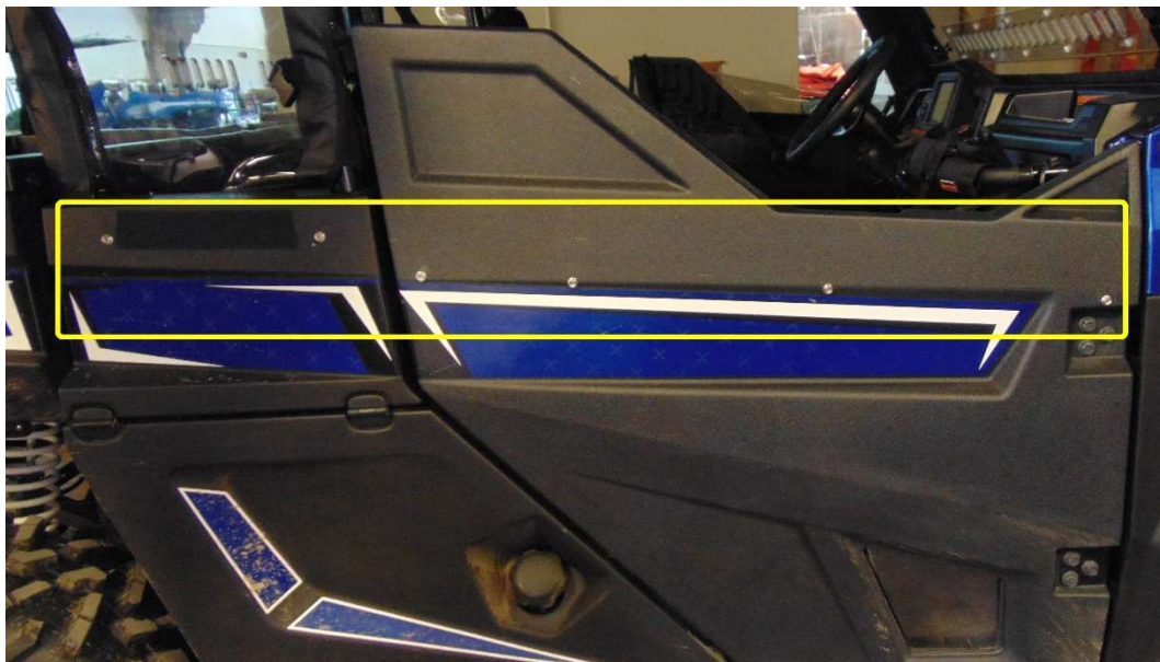
Figure 12: After installing the doors on the UTV you can then use the female end of the snaps attached to the door kit to determine the best spot for male end on the UTV. Mark the area on which you will install your snap, use a Phillips head screw driver to twist it into place.
