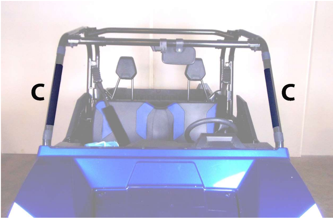
Figure 3: Shows placement of 14" Velcro strips C.
