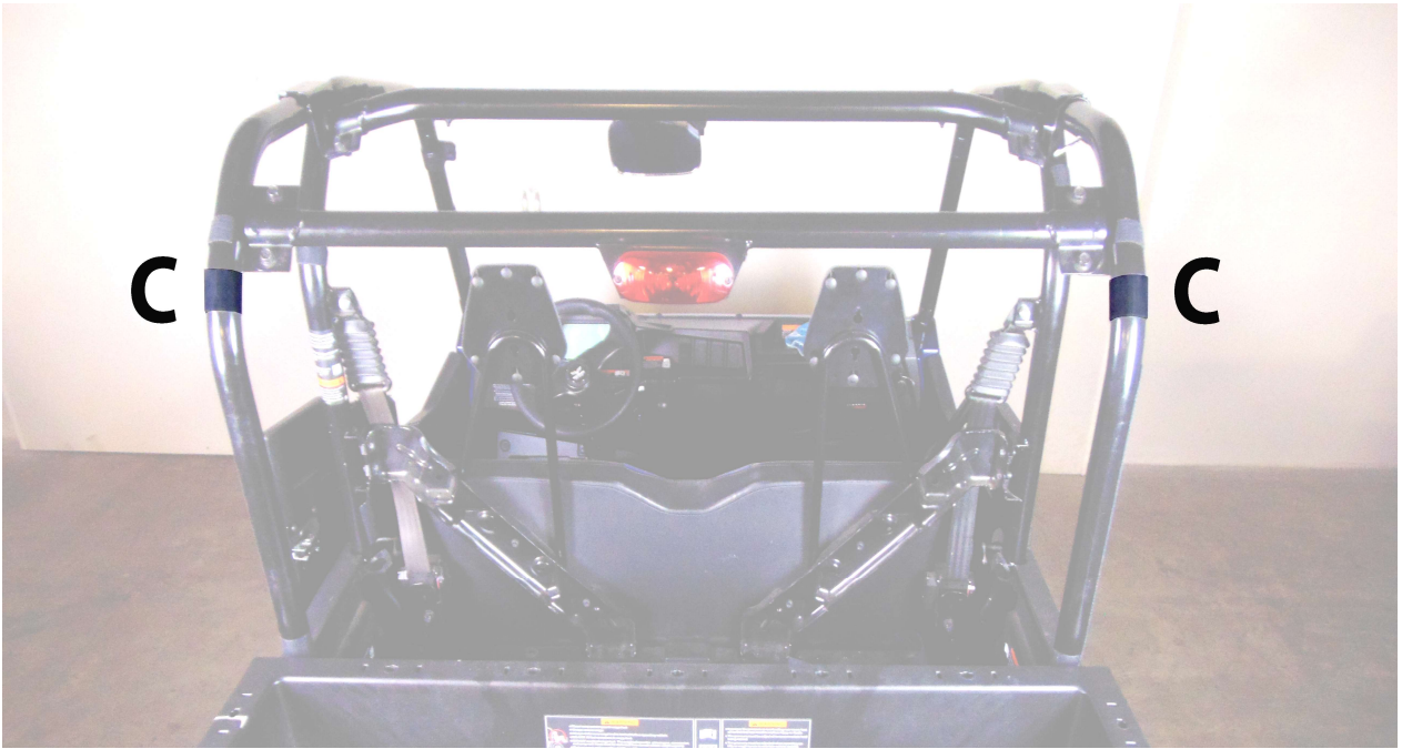
Figure 3: Shows placement of 6" Velcro strips C.
