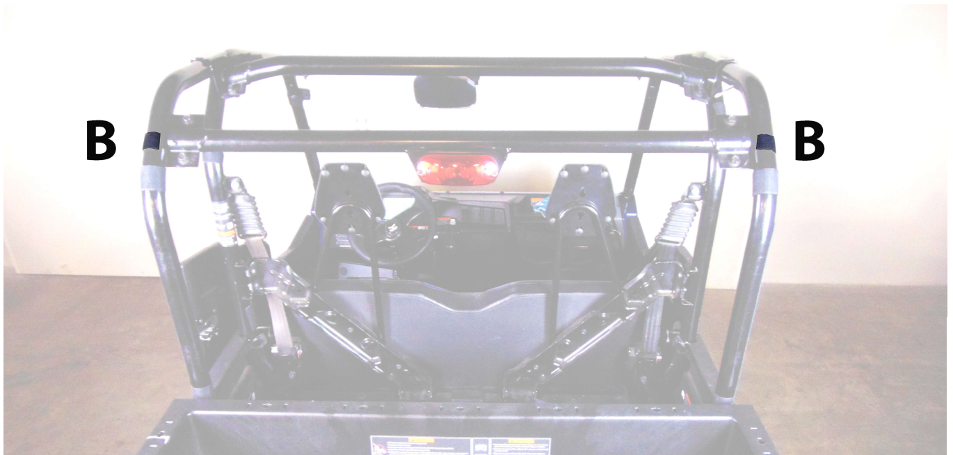
Figure 2: Shows placement of 3" Velcro strips B.
