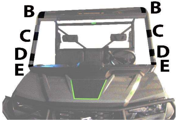
Figure 6: Shows placement of 6" Velcro strips B. Wraps these strips around the roll bars on passenger and drivers side.
