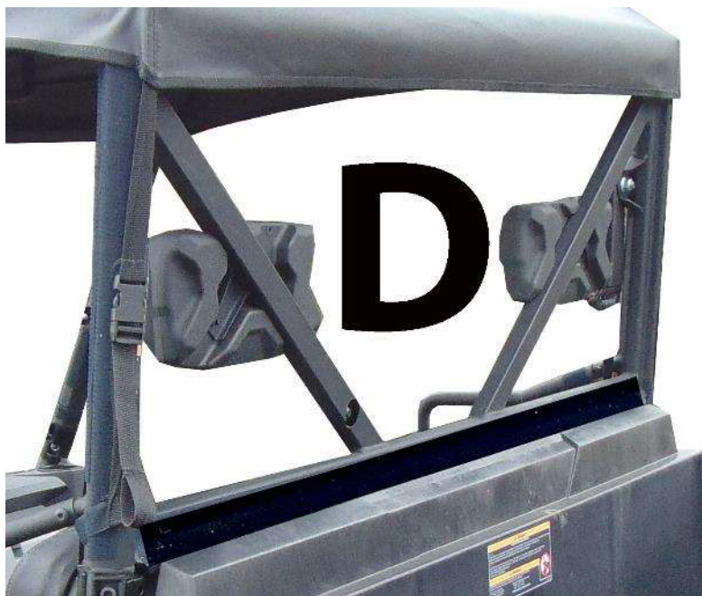
Figure 3: Shows placement of Velcro strip D.
