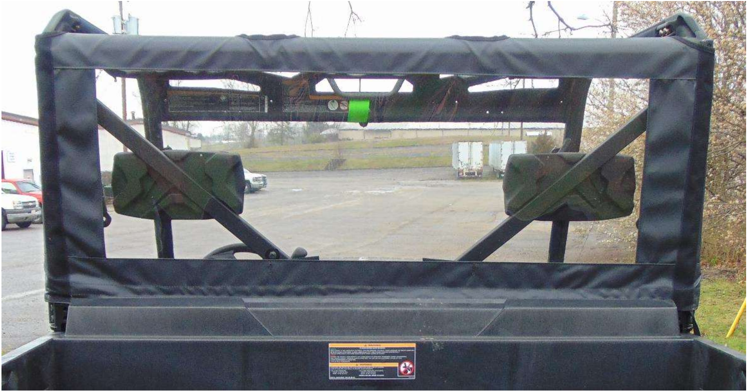
Figure 4: Upon completion of installation your back panel should be tight across the back of the UTV.
