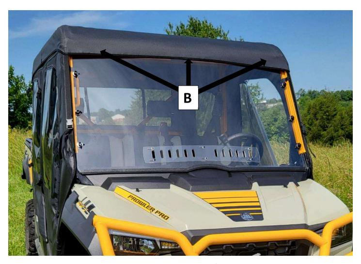
OPTIONAL-Windshield must be installed before completing this step. Unwrap the front two double-sided straps. Remove the adhesive backing from the 50" adhesive hook strip. Adhere the strip to the top of the windshield corresponding to the sewn-in loop in the visor.
