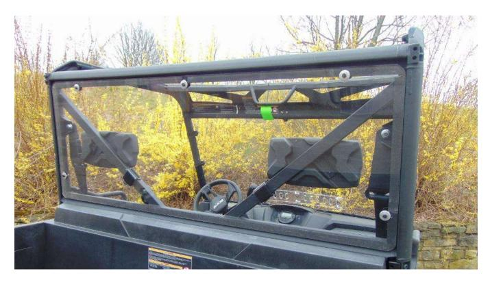
**Step 4:** The CC Clamps use the roll cage inset for connection. When installed properly, the back edge of the clamp attaches to the outside edge of the roll bar insert as shown below.
