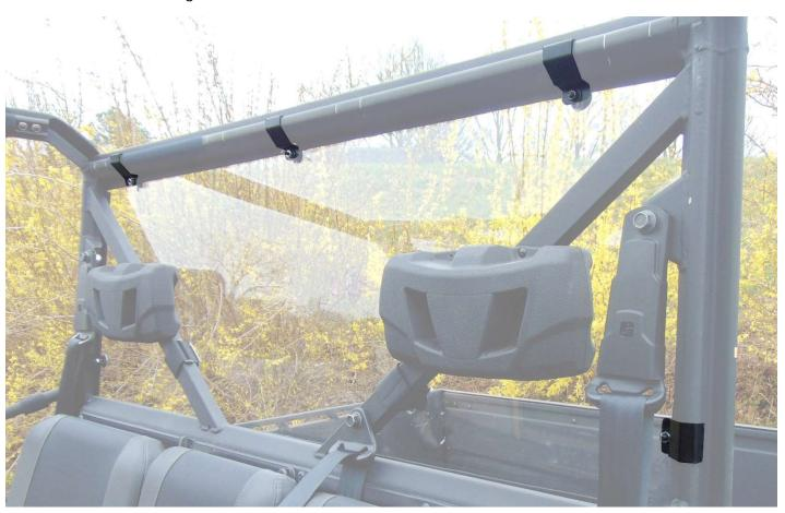
**Step 5:** After installing all four CC clamps, remove the protective plastic paper from the outside of the back panel.
