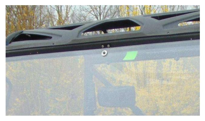
**Step 4:** Install C Clamps, hook clamp on to the pro-fit cage and push the flat part towards the windshield. Take a wingnut and slide it over the bolt, then slide the neoprene washer over the bolt and insert through the outside of the lexan windshield and though the hole in the C Clamp. Secure with small washer and lock nut.
