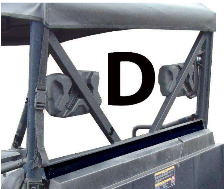
Figure 3: Shows placement of Velcro strip D.
