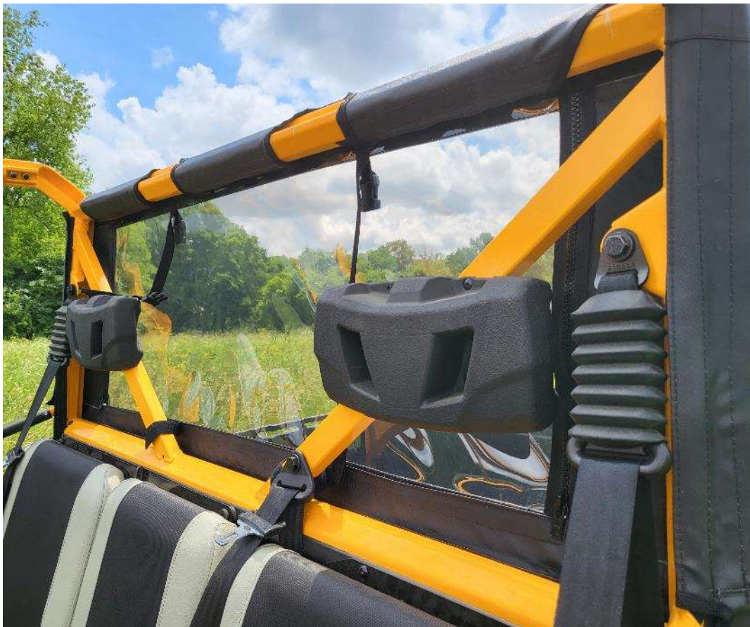
Figure 4: Upon completion of installation your back panel should be tight across the back of the UTV.
