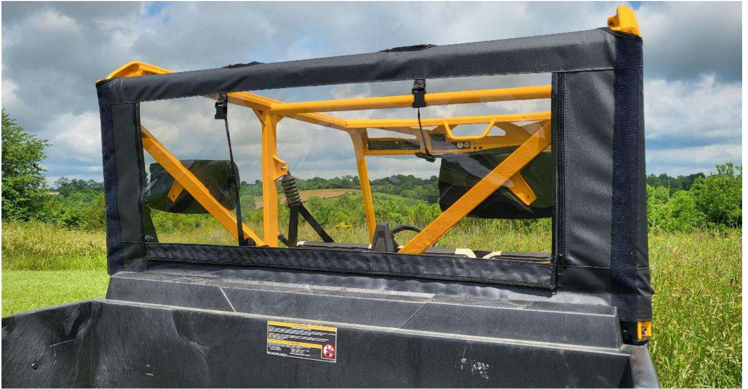
Figure 4: Upon completion of installation your back panel should be tight across the back of the UTV.
